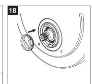
Reinstall the inner white temperature range control ring.
