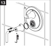
Reinstall the temperature control handle and escutcheon making sure the temperature override button is on top and the handle is set at 6 o'clock.
