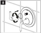
Set the volume control/diverter handle and escutcheon at 12 o'clock and place on the top stem and nipple. Rotate the escutcheon clockwise to secure the assembly to the plate.
