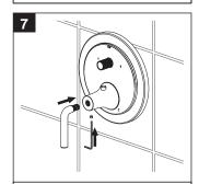
Align the handle at 6 o' clock position and slide handle into escutcheon and secure with set screw.
