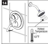
The valve maximum temperature is set at 107°F. Should your customer like to change this go to step #15. If not go to step #20.
