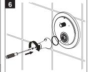
Slide on temperature control escutcheon engaging the stem making sure the temperature override button facing straight up. Secure with screw.
