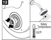
Rotate the cartridge stem to adjust safety temperature. Rotate clockwise to reduce temperature while rotate counterclockwise to increase temperature. Once the temperature is 100°F go to step #13.
