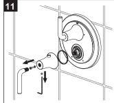
Turn off the water supply. Remove temperature control handle and escutcheon.
