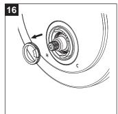
Remove the inner white temperature range control ring.
