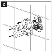
Turn off the water supply and remove the mud guard.
