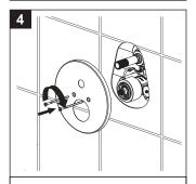
Install escutcheon with 2 screws. Do not overtighten the screws.
