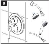
Turn on the water supply. Remove all shower heads and/or hand showers. Turn the volume control/diverter handle to each function to flush the system.
