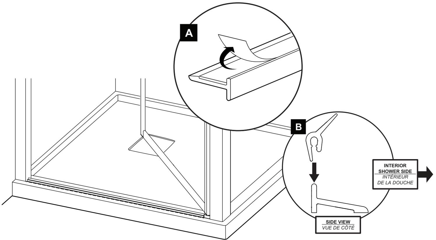
CUT THE WALL JAMB CAP ACCORDING TO THE DOOR'S CONFIGURATION. IF SPACERS WERE REQUIRED, CUT THE CAPS BASED ON THE NUMBER OF SPACERS USED IN THE INSTALLATION. IF NO SPACERS WERE REQUIRED, CUT THE CAP TO THE MINIMUM.
