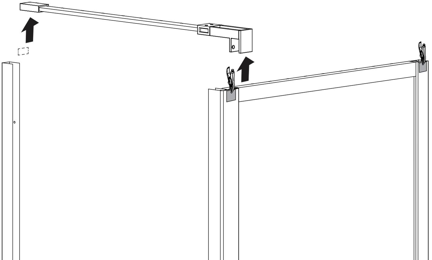
**PLACE THE WALL MOUNT ON THE PREVIOUS MARK AND MARK THE HOLE LOCATION /
