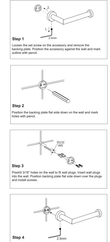
Slide the accessory onto the backing plate and tighten the set screw using Allen key provided.
