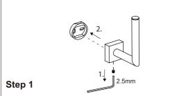
Loosen the set screw on the accessory and remove the backing plate. Position the accessory against the wall and mark outline with pencil.
