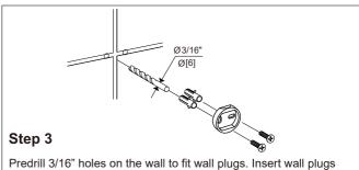
into the wall. Position backing plate flat side down over the plugs and install screws.
