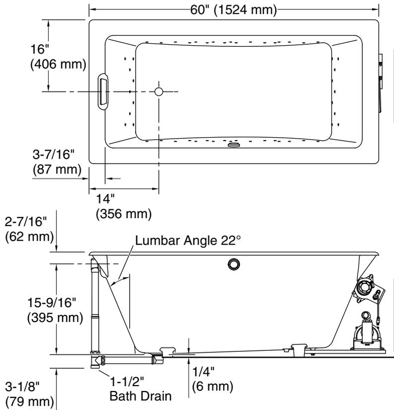
No change in measurements if connected with drain illustrated. (K-7169AF)
