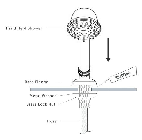
Other end of Hose to connect to Spout Diverter Valve
